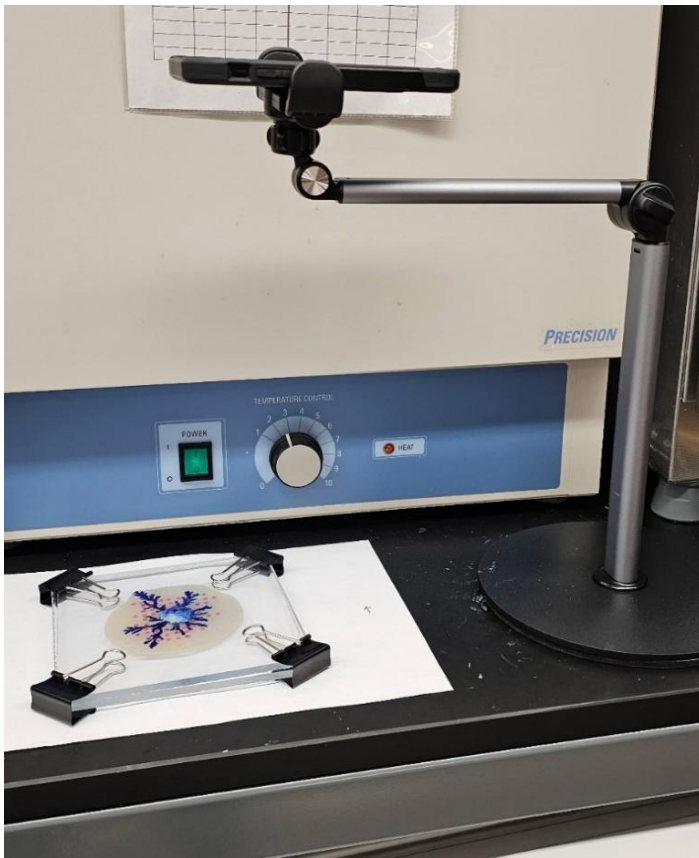
Figure 1. Experimental setup for Hele-Shaw cell.
